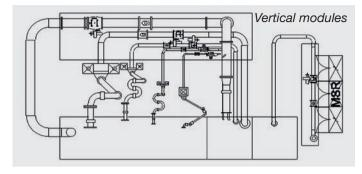
All 5 modules use a common basin located below the hall floor. Each module has a loading arm with piping in stepped nominal diameters from DN 50 to DN 400 and an integrated sensory system. The adjustment of the operating points is implemented here too using plunger valves.
